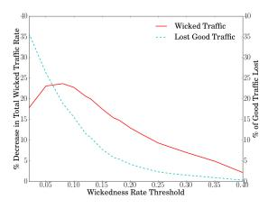
Figure 8: The reduction in wicked traffic and the loss of legitimate (good) traffic when blacklisting all ASes of degree < 170.
