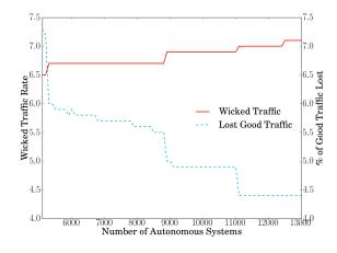
Figure 9: Change wicked traffic and loss of legitimate traffic over time as the network grows from 5 000 to 13 000 ASes. The wicked traffic rate is the percentage of all traffic that is wicked.
