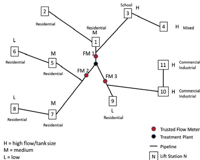
**Fig. 1 – Reference wastewater facility (trust anchors placed in flow meters are in red).**(For interpretation of the references to color in this figure legend, the reader is referred to the web version of this article.)
