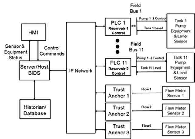
**Fig. 2 – Reference wastewater facility hardware.**
