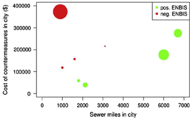
Fig. 4 – Comparison of the number of sewer miles with the costs of deploying countermeasures for the eight representative cities. The size of a point indicates the magnitude of the net benefit (or cost) of deploying countermeasures.
