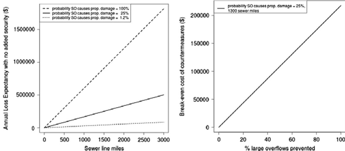
Fig. 3 – The expected loss  $ALE_0$  for a utility expressed as a function of the length of sewer lines managed, shown for varying probabilities of experiencing property damage (left); the breakeven costs of countermeasures expressed as a function of the percentage of large overflows prevented through improved detection (right).
