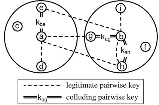
**Figure 1. Example key-swapping collusion attack between attacker nodes  $a$  and  $b$ .**
